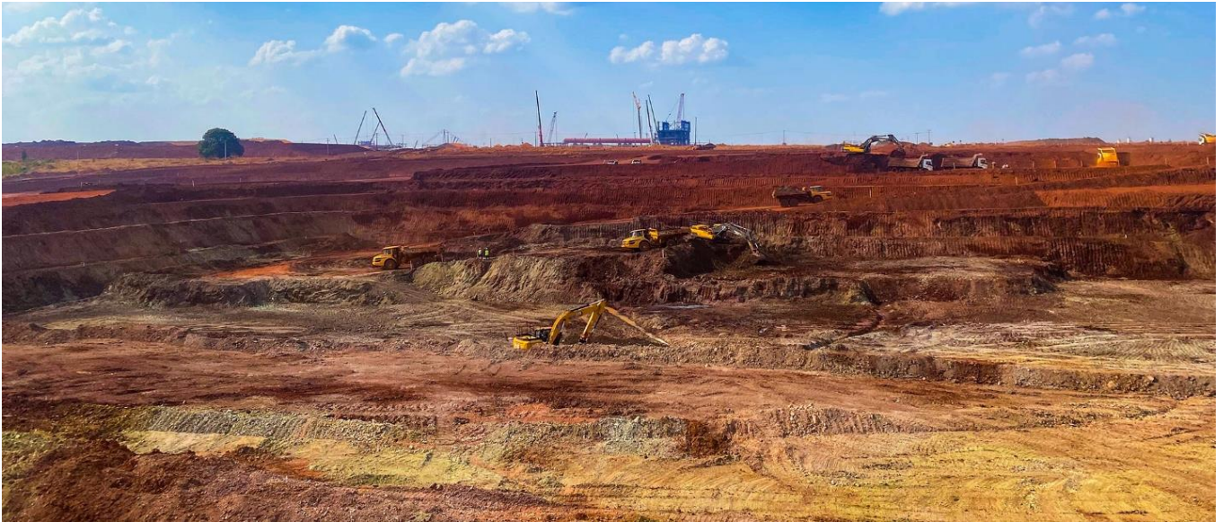
Mining at the Pequizeiro pit showing the excavators currently in the high-grade transition zone. The processing plant is shown in the background approximately 500m from the mine.
