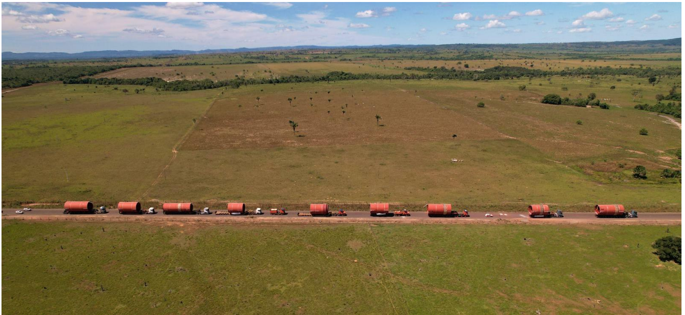
Figure 1: One of the convoys carrying the kiln sections making its way to site. The kiln arrived in the Port of Outeiro in northern Brazil and travelled by barge up the Araguaia River to Araguatins before being transported to site by road.
