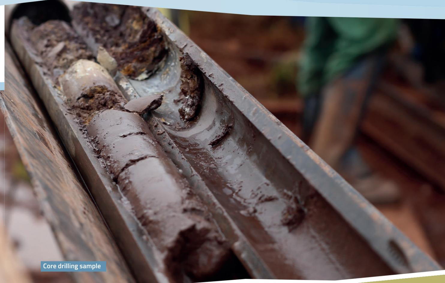
Core drilling sample
