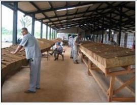
Logging and sampling of large diameter cores
