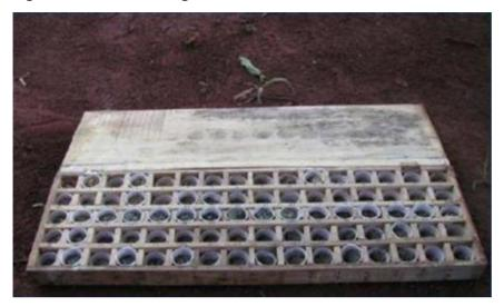
Sample lithology was described using the RC cuttings. In total, the project geologists differentiated 13 lithologies, which are listed in Table 10-3 (including the corresponding codes). The HZM technical team elected to update the nomenclature of the weathering units so that they are in alignment with HZM's other projects (refer to Section 7.4 for details).
