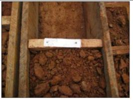
Large diameter coring operations – depth markers in core boxes
