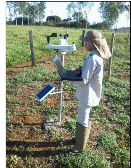
Figure 5-4 Local meteorological monitoring station
