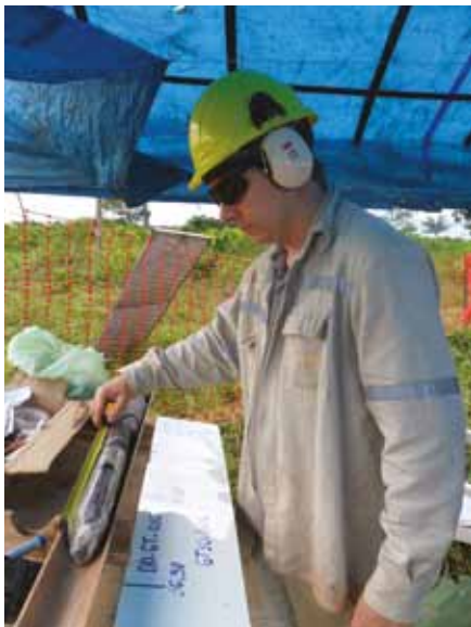
Field technician measuring core recovery. Part of the 3rd Phase drill programme.
