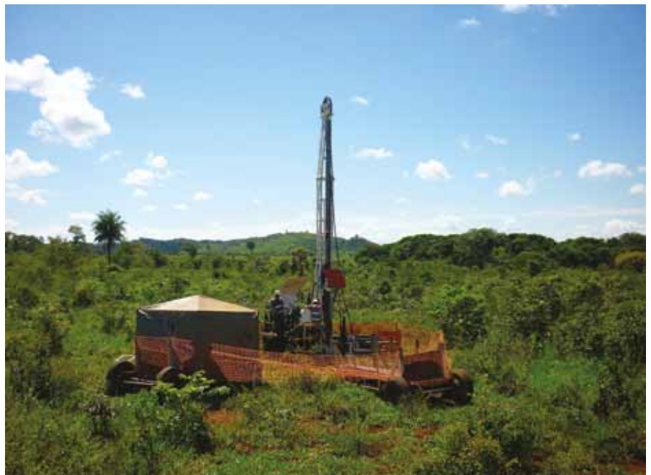
HQ diamond drill rig in action as part of the 3rd Phase drilling programme.
