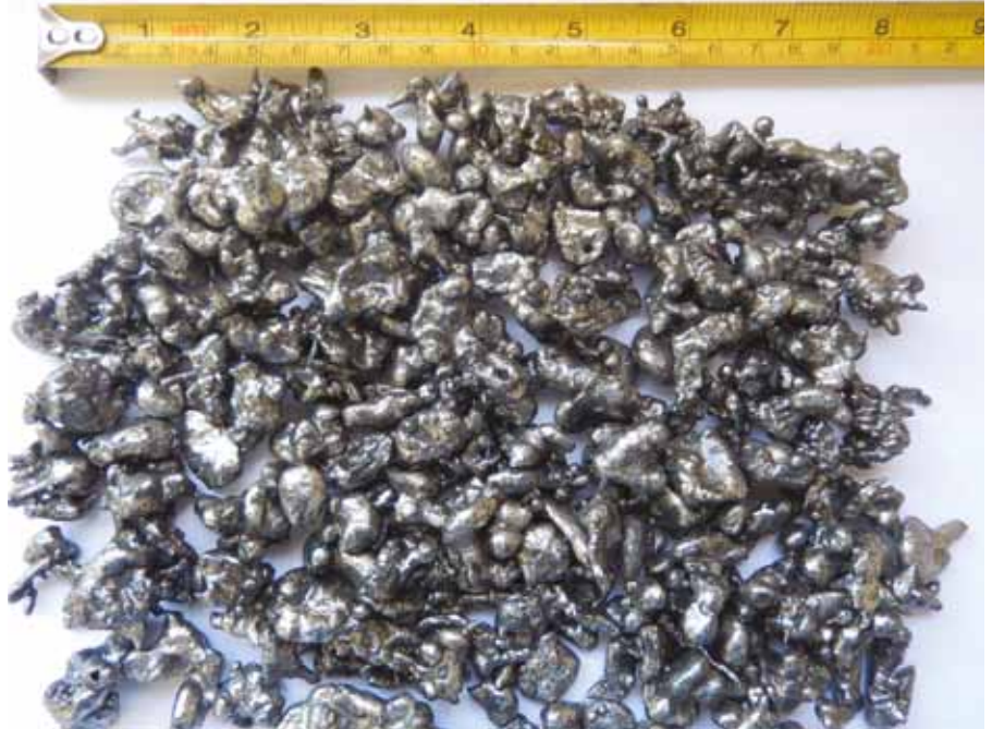
Ferronickel prills grading 20% Ni produced at Morro Azul facility.
