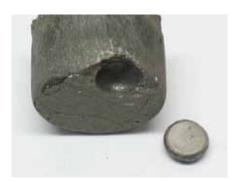
Sample of ferronickel produced by XPS from blended ore from Araguaia grading 34.3% Ni and 63.9% Fe
