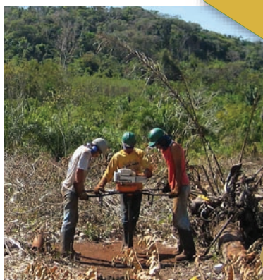
Auger drilling - Lontra, Brazil Jan 2008
