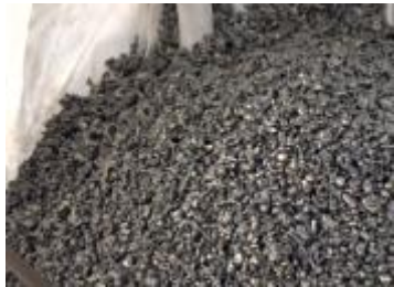
HZM FeNi 30 produced at the Morro Azul RKEF facility in Brazil – June 2015
